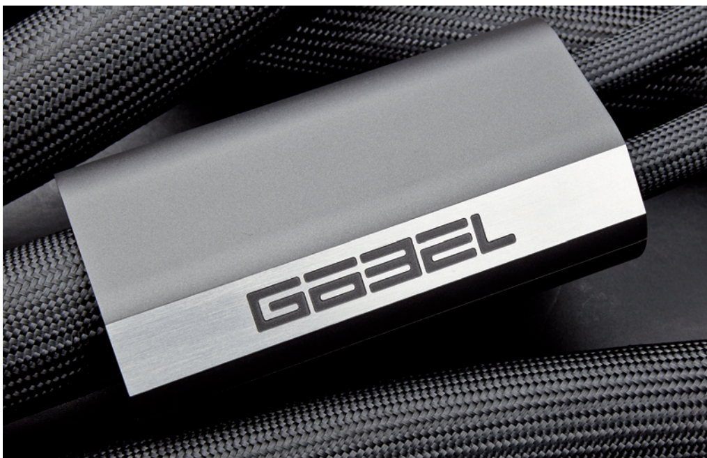
The splitbox really only has the task of covering the junction of the actual wiring to the connectors. But due to their weight they also stabilize the relatively light cable thereby preventing any microphonic effects
